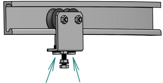
Hang the door to the runners using the door brackets
