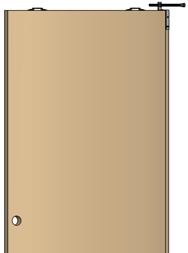
NOTE: before fitting the door brackets check and ensure the top face is perfectly at right angles to the vertical door axis
